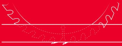
1. Remove the battery from the circular saw, and adjust the cutting depth so that one to two teeth are protruding past the timber.
