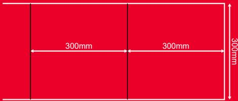
1. Measure & mark two 300mm squares on the timber work piece. Clamp securely and cut along the lines using a circular saw.
