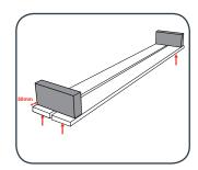
4 Place seat bases into position and attach 2 hinges to each using 4 x 20mm screws in each hinge.
