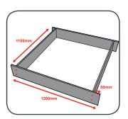
2 Cut the treated pine decking boards to 1200mm long and screw 2 to each end of the box using 40mm screws and drill driver. Use 2 screws at both ends of each decking board. Have a gap of 10mm between boards and ensure the screw heads are flush with the top of the boards.
