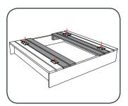
5 Cut 90 x 45mm pine at 420mm and screw to 2 pine decking boards, in-setting the timber 50mm from the edge. Ensure a 10mm gap is left between the boards as shown to the right. Create 2 of these.
