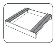
3 Cut the treated 90 x 45mm pine at 190mm and screw to 2 pine decking boards with a 10mm gap as shown above. Use 2 screws at both ends of each decking boards.
