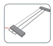
6 Screw 4 more hinges to the under side of the seat back rest.
